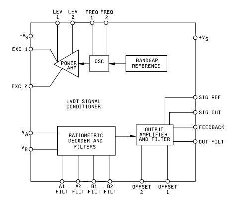
FIGURE 2. Block diagram.
